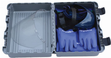
Cryogenic safety equipment
